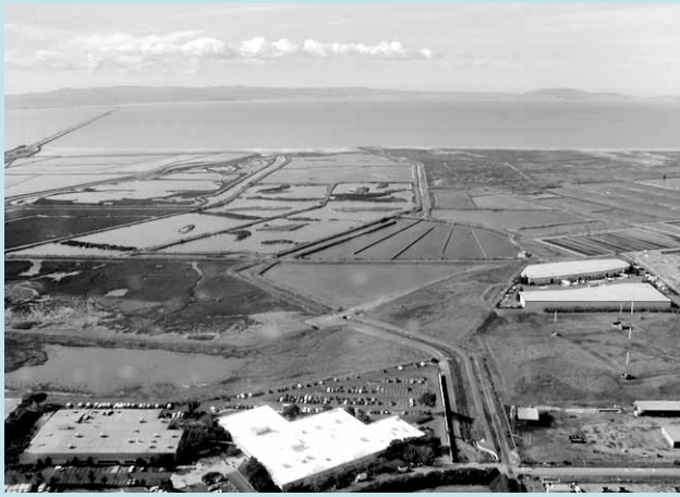
The Hayward Marsh expansion project created fresh and brackish water marsh basins that include wildlife islands for waterbirds and a pickleweed marsh for the endangered salt marsh harvest mouse. The marsh system utilizes secondary treated wastewater and storm runoff.
